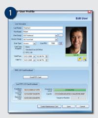
**Manage User Profile:** The E-Plex FIPS 201 software allows you to add and maintain users, import their photos, and check the status of Smart Cards.
